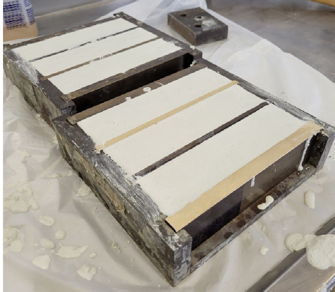
Figure 1.1 – Casting of specimens using the Piazza Stone mortar mix
