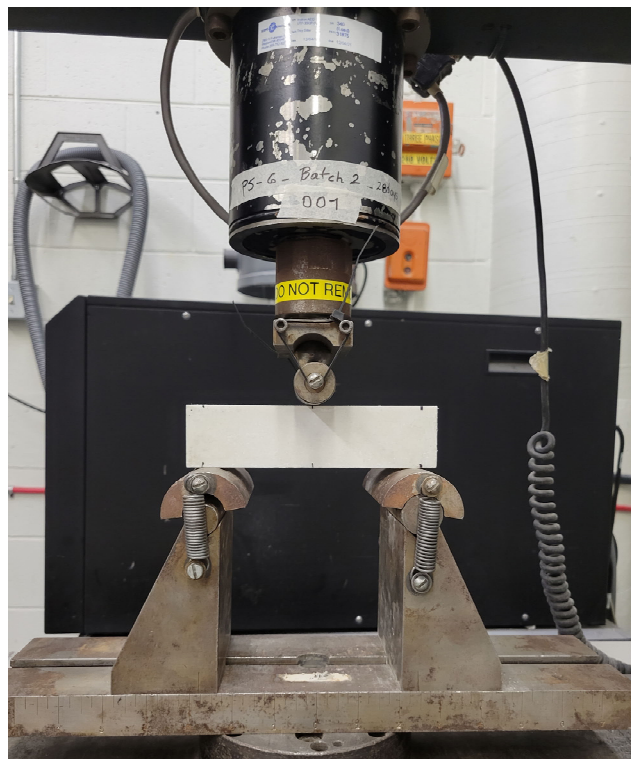
Figure 1.2 – Flexural strength test setup
